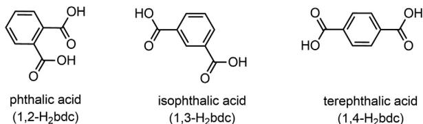
**Fig. 1.** The structural formulae of benzenedicarboxylic acids.
