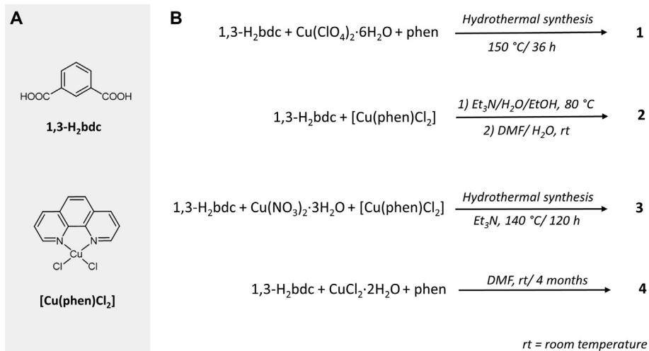
**Fig. 10.** (A) Structures of the building blocks 1,3-bdc and [Cu(phen)Cl<sub>2</sub>] and (B) schematic representation of reactional conditions for the syntheses of **1** and **2**, and the CPs previously reported **3** and **4** [17,18].
