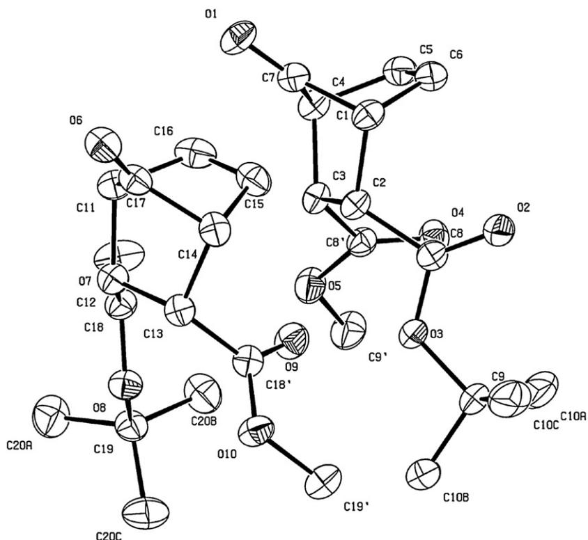
Fig. 1. X-ray structure of *t*-butyl methyl 7-oxo-5-norbornene-2-*endo*,3-*endo*-dicarboxylate (**8a**) showing both the *R,S* and *S,R* enantiomers.
