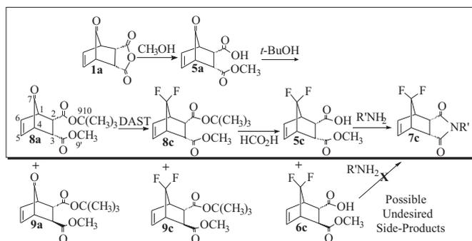
**Scheme 2.** Synthetic scheme for the preparation of 7,7-difluoronadic acid ester **5c** and the corresponding polyimides **7c**. The large rectangular box includes the critical precursors along this synthetic pathway, while those compounds lying outside the box are possible undesired side-products with inverted configuration at C<sub>3</sub>.
