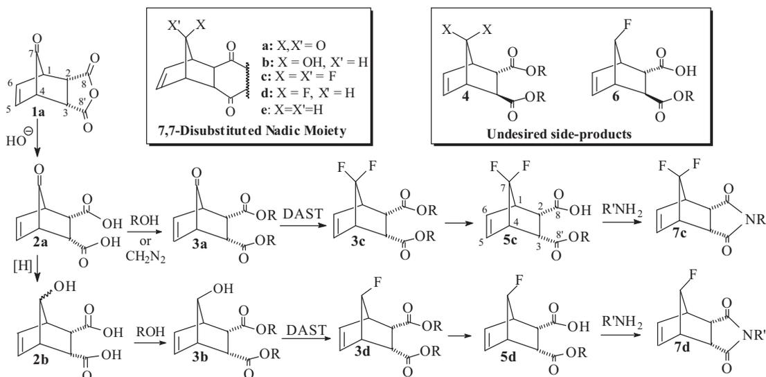
**Scheme 1.** Proposed scheme for the preparation of 7,7-difluoronadic and 7-fluoronadic acid esters **5c** and **5d**. Undesired *endo,exo* side-products **4** and **6** will not lead to imide **7**.
