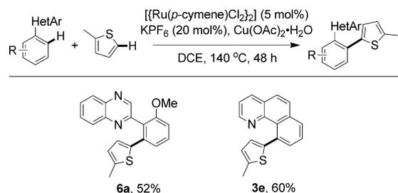
**Scheme 4.** Ru-catalyzed direct heteroarylation of N-heteroarene-substituted arenes by double C–H activation. Reaction conditions: biaryl (0.25 mmol), 2-methylthiophene (0.75 mmol),  $[\{\text{Ru}(p\text{-cymene})\text{Cl}_2\}_2]$  (5 mol %),  $\text{KPF}_6$  (20 mol %),  $\text{Cu}(\text{OAc})_2 \cdot \text{H}_2\text{O}$  (2.0 equiv), and DCE (2 mL) at 140 °C for 48 h.
