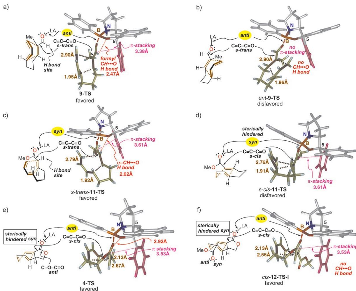
**Figure 2.** PCM B3LYP/6-31G(d) calculated transition-state structures for intramolecular Diels–Alder reactions catalyzed by oxazaborolidinium **1b**·H<sup>+</sup>. a) and b) TSs for **9**; c) and d) TSs for **11**; e) TSs for **4**; f) TSs for **12**.
