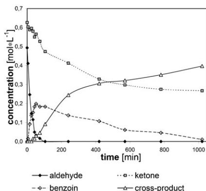
**Fig. 3** Direct observation of the reaction progress via  $^1\text{H-NMR}$ -spectroscopy. The reaction was performed using 0.5 mmol aldehyde, 0.65 mmol ketone, 0.5 mmol *i*-Pr<sub>2</sub>NEt and 0.01 mmol catalyst **5** in 1 mL THF-*d*<sub>8</sub> at room temperature.
