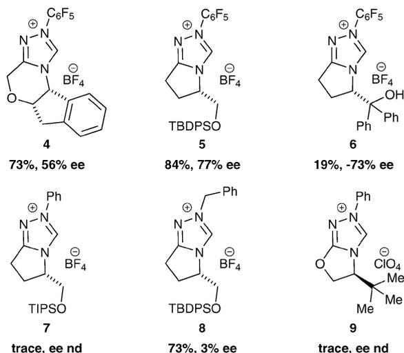
**Scheme 1** Catalyst screening result of the reaction between furfural (**1a**) and trifluoroacetophenone (**2a**).
