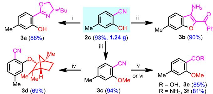
**Scheme 3** Gram-scale synthesis of **2c** and its synthetic transformations. Reaction conditions: i) (*S*)-2-Amino-3,3-dimethylbutan-1-ol, ZnCl<sub>2</sub>, PhCl, 131 °C, 72 h; ii)  $\alpha$ -Bromoacetophenone, K<sub>2</sub>CO<sub>3</sub>, acetone, reflux, 8 h; iii) MeI, K<sub>2</sub>CO<sub>3</sub>, DMF, 60 °C, 5 h; iv) (+)-Fenchol, KO<sup>t</sup>Bu, dioxane, rt, overnight; v) 34% aq. KOH, EtOH, 80 °C, overnight, for **3e**; vi) KOH(s), <sup>t</sup>BuOH, 60 °C, overnight, for **3f**.
