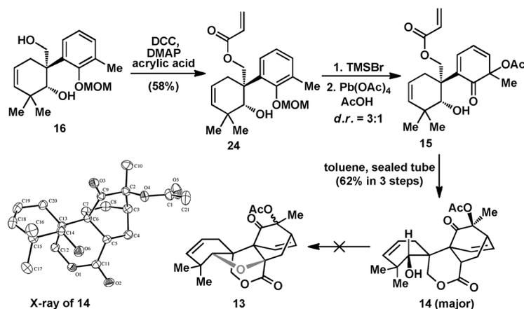
**Scheme 3.** Construction of the core structure of Maoecrystal V through an IMDA. Thermal ellipsoids are scaled to the 50% probability level.
