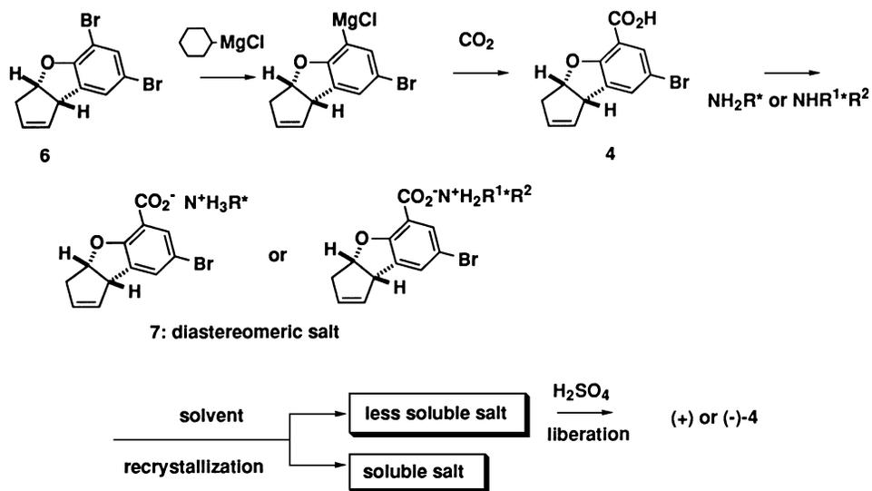
Scheme 3. Preparation and resolution of the carboxylic acid 4
