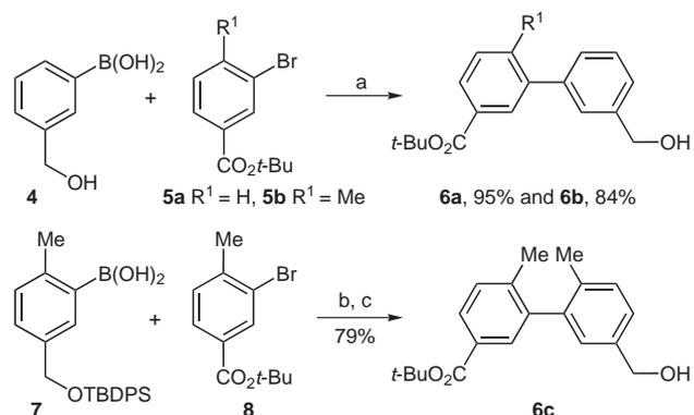
**Scheme 4** Reagents and conditions: a) Pd(PPh<sub>3</sub>)<sub>4</sub> (2 mol%), aq Na<sub>2</sub>CO<sub>3</sub>, THF, 80 °C, 18 h; b) Pd(OAc)<sub>2</sub> (2 mol%), S-Phos (5 mol%), aq K<sub>3</sub>PO<sub>4</sub>, toluene, 90 °C, 16 h; c) TBAF, THF, 0 °C to r.t., 4 h, 95%.
