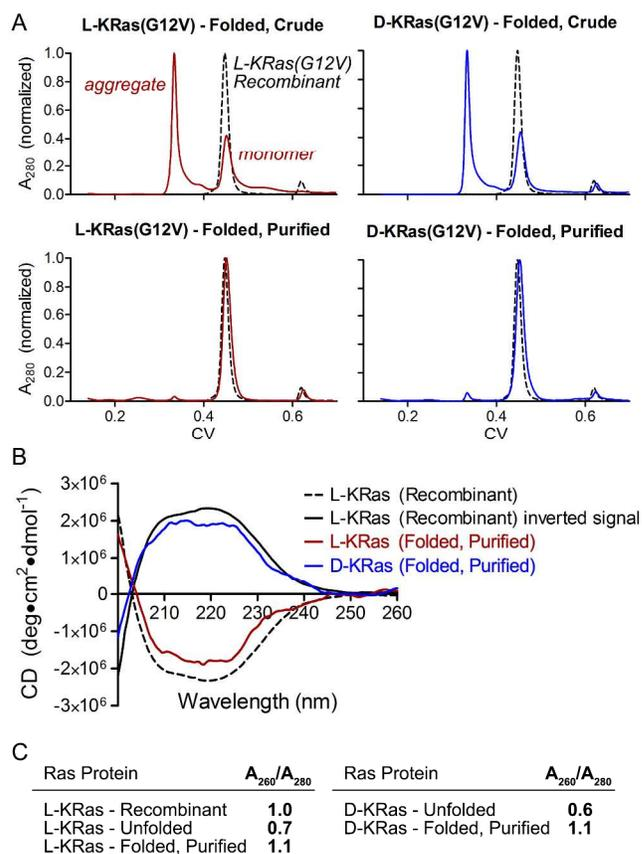
**Figure 4:** Folding analysis of synthetic proteins. A) Crude gel filtration traces and purified synthetic all L- and all D-KRas(G12V) after folding with GppNHp; B) Circular dichroism analysis of folded and purified synthetic proteins and recombinant KRas(G12V); C) Comparison of  $A_{260}/A_{280}$  values for synthetic proteins and recombinant KRas(G12V).
