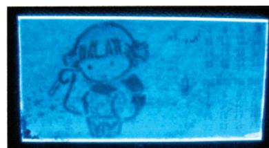
**Figure 5.** PL image prepared by irradiation of a film of poly[ethoxy(methyl)silylene-*p*-phenylene] containing (trimethylsilylethynyl)pyrene in air.
