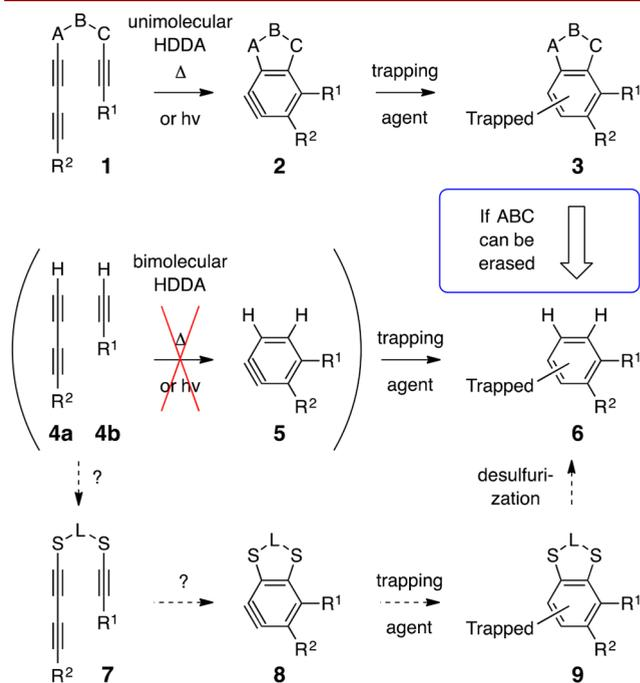
**Figure 1.** Hypothesis driving this study: Temporary tethering of a 1,3-diyne to a diynophile (cf. **7**) to support intramolecular HDDA cyclization (**1** to **3** via **2**, or **7** to **9** via **8**), and removal of the tether (**3** or **9** to **6**), allows for an otherwise infeasible intermolecular HDDA reaction (cf. **4a** + **4b** to **6** via **5**).
