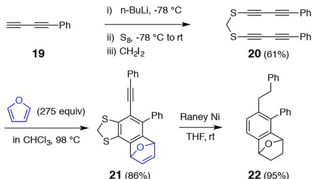
**Figure 3.** Alternative synthesis of tetrayne substrates and an example of external benzyne trapping.
