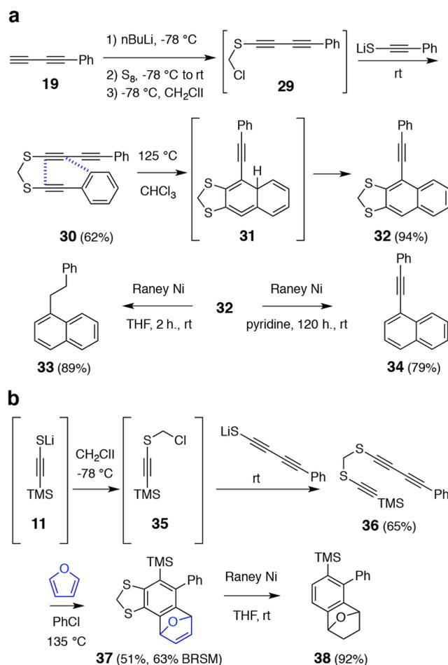
**Figure 5.** (a) Phenyl-substituted triyne **30** is diverted to a TDDA cycloisomerization pathway. (b) When the TDDA reaction is not possible, triyne **36** undergoes the HDDA reaction in the normal fashion.
