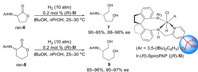
To evaluate various chiral catalysts, we chose racemic  $\alpha$ -phenylamino  $\gamma$ -butyrolactone (**6a**) as a model substrate. Ir-SpiroPAP catalysts **5**,<sup>12</sup> which were developed by our group, were found to efficiently catalyze the desired hydrogenation reaction to afford chiral *N*-phenyl-2-aminobutane-1,4-diol (**7a**, Scheme 2). Catalyst (*R*)-**5c** (79% ee), which has a 3,5-di-*tert*-
