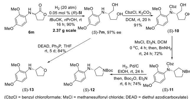
material for constructing chiral 3-arylamino 1-aza/oxocycloalkanes, which are present in many chiral pharmaceuticals.<sup>15</sup> Specifically, selective protection of the arylamino group of (S)-**7m** with benzyl chloroformate generated 1,4-diol (S)-**10** in 91% yield. Activation of the hydroxyl groups of (S)-**10** with methanesulfonyl chloride (MsCl) and subsequent treatment with benzyl amine ( $\text{BnNH}_2$ ) gave 3-arylamino-1-pyrrolidine
