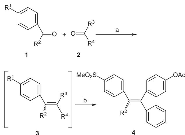
**Scheme 1** Reagents and conditions: (a) Zn, TiCl<sub>4</sub>, THF, reflux 4.5 h; (b) AcCl, TEA, Et<sub>2</sub>O, 25 °C, 1.5 h.
