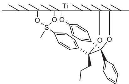
**Figure 2** Proposed mechanism for stereoselective Z-olefin formation as illustrated for (Z)-1-(4-hydroxyphenyl)-1-phenyl-2-(4-methylsulfonylphenyl)pent-1-ene: A surface induction pattern involving metallic titanium and the polydentate pinacol intermediate.<sup>1,4</sup>
