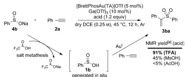
**Scheme 2.** One-pot synthesis of vinyl sulfone **3ba** from bench-stable sodium benzenesulfinate (**4b**). [a] Yield determined by <sup>1</sup>H NMR spectroscopy with 1,3,5-trimethoxybenzene as the internal standard.
