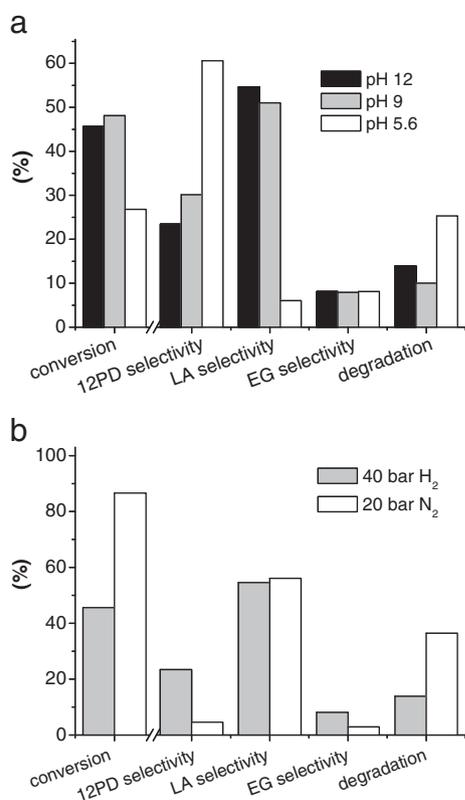
**Fig. 3.** <sup>a</sup> Effect of pH on glycerol conversion and selectivity. Reaction conditions: 5 mol% Pt/CaCO<sub>3</sub>, 5 mL aqueous reaction mixture (100 mM glycerol, 100 mM BA, variable pH), 200 °C, 40 bar H<sub>2</sub>, 18 h, 800 rpm; <sup>b</sup> Effect of hydrogen pressure vs. inert atmosphere. Reaction conditions: 5 mol% Pt/CaCO<sub>3</sub>, 5 mL aqueous reaction mixture (100 mM glycerol, 100 mM BA, pH 12), 200 °C, 40 bar H<sub>2</sub> or 20 bar N<sub>2</sub>, 18 h, 800 rpm.
