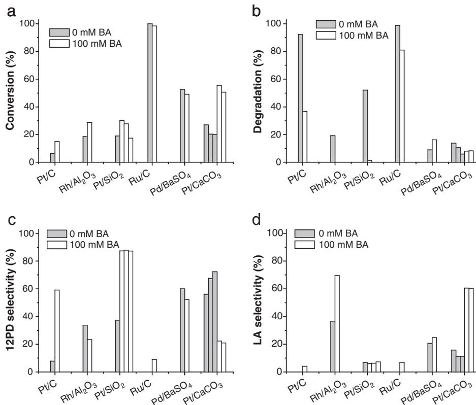
**Fig. 1.** The influence of BA on <sup>a</sup> conversion; <sup>b</sup> degradation; <sup>c</sup> 12PD-selectivity and <sup>d</sup> LA selectivity. Some reactions were performed in duplicate or triplicate in order to establish the error margin. Reaction conditions for the respective catalysts are given in Table S1, Supplementary Data.
