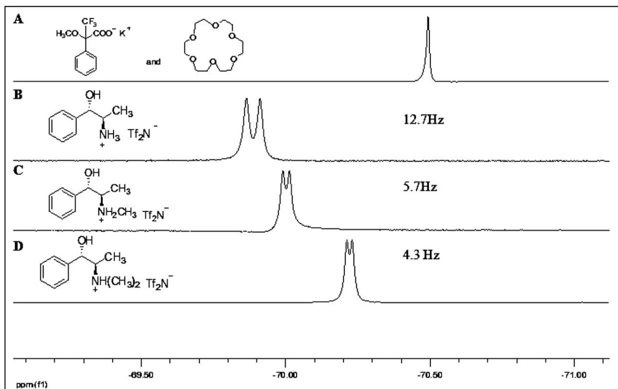
Fig. 4.  $^{19}\text{F}$ -NMR ( $\text{CDCl}_3$ ) spectra of potassium Mosher's salt (A), potassium Mosher's salt with (1*S*,2*R*)-NorHEph $\text{TF}_2\text{N}^-$  as chiral selector (B), potassium Mosher's salt with (1*S*,2*R*)-HEph $\text{TF}_2\text{N}^-$  as chiral selector (C), and potassium Mosher's salt with (1*S*,2*R*)-MeHEph $\text{TF}_2\text{N}^-$  as chiral selector (D).
