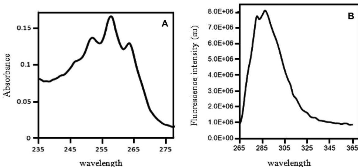
Fig. 5. (A) UV-vis spectrum of 10 mM MeHEphTf<sub>2</sub>N in methanol. (B) Fluorescence of neat MeHEphTf<sub>2</sub>N excited at 260 nm with front-face illumination.
