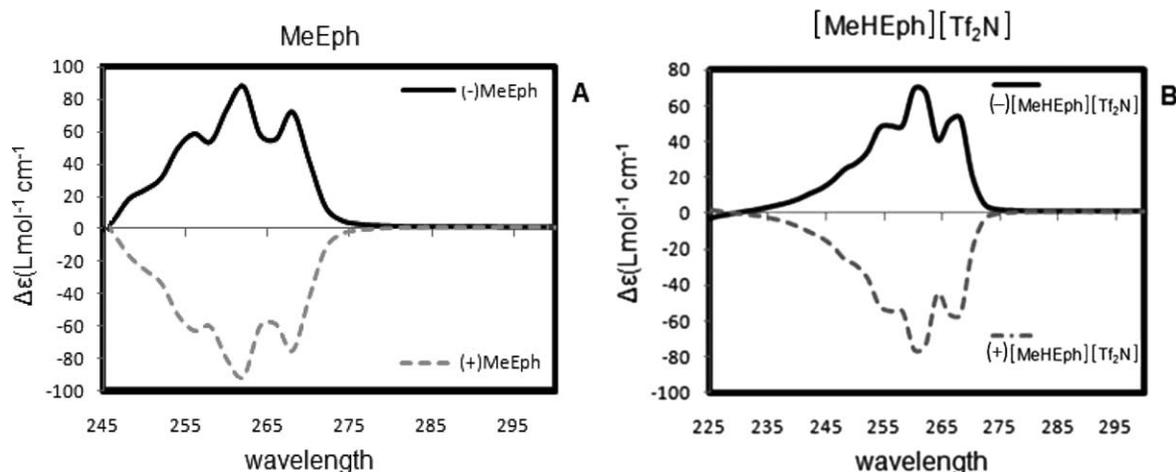
**Fig. 2.** Circular dichroism of enantiomers (+ and -) of (A) 10 mM MeEph and (B) 10 mM MeHEphTf<sub>2</sub>N in methanol.
