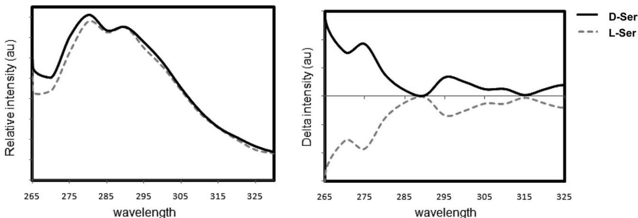
Fig. 8. Fluorescence spectrum of 10  $\mu\text{M}$  serine in 30 mM aqueous solution with [NorHEph][Tf<sub>2</sub>N] as chiral selector.
