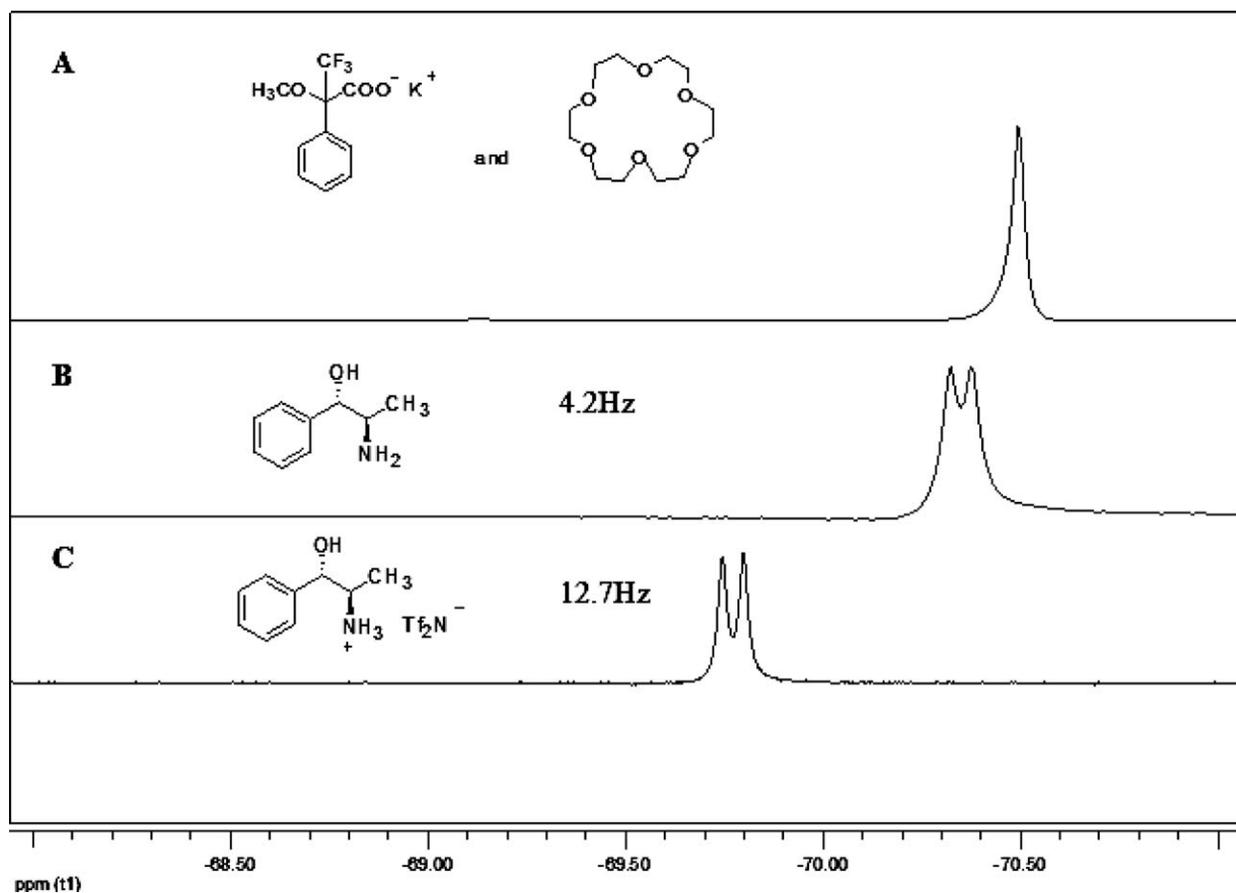
Fig. 3.  $^{19}\text{F}$ -NMR ( $\text{CDCl}_3$ ) spectra of potassium Mosher's salt (A) without chiral selector and with (B) (1*S*,2*R*)-NorEph and (C) (1*S*,2*R*)-NorHEph $\text{TF}_2\text{N}^-$  chiral selector.
