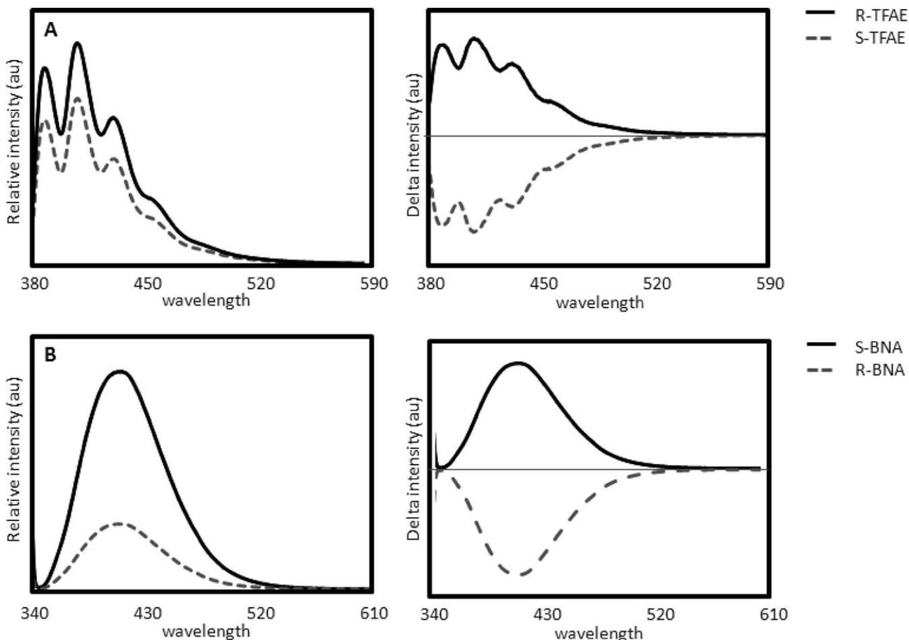
**Fig. 7.** A. Fluorescence spectrum of 10  $\mu$ M TFAE in aqueous solution with 30 mM [NorHEph][Tf<sub>2</sub>N] as chiral selector. B. Fluorescence spectrum of 10  $\mu$ M BNA in aqueous solution with 30 mM [MeHEph][Tf<sub>2</sub>N] as chiral selector.
