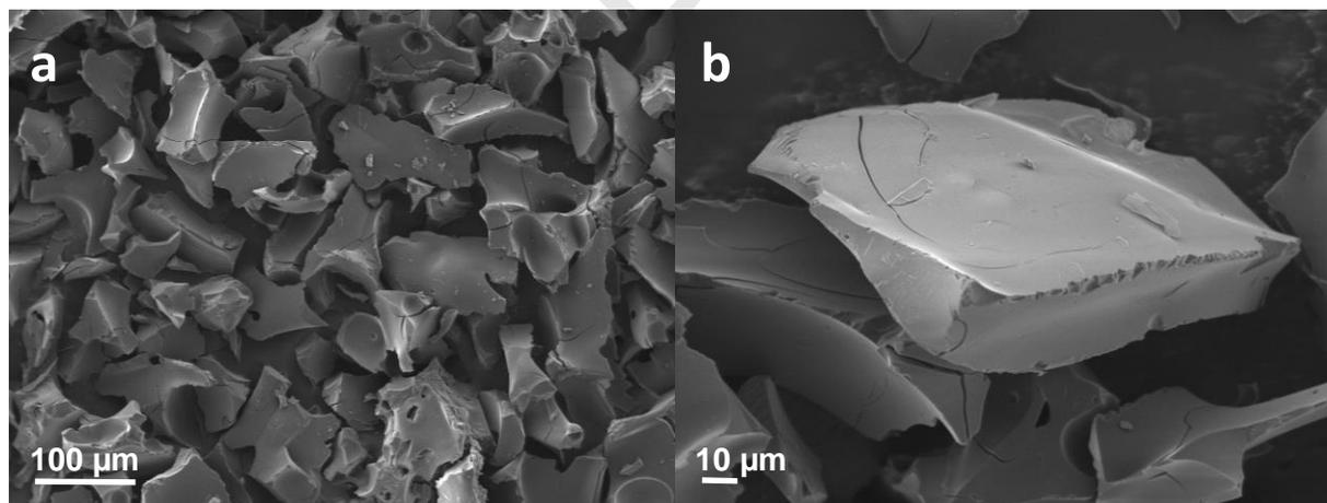
**Figure 1.** SEM images of the Starbon®450-SO<sub>3</sub>H catalyst powder obtained at different magnifications, (a) 180X and (b) 650X.
