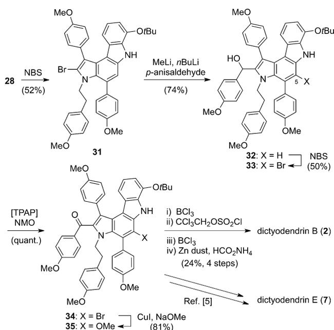
**Scheme 6.** Total synthesis of dictyodendrins B and E. NMO = *N*-methylmorpholine *N*-oxide, TPAP = tetrapropylammonium perruthenate.
