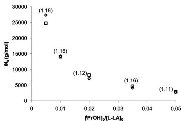
**Fig. 8** Plot of  $M_n$  vs. alcohol-to-metal ratio for the polymerisation of L-LA (complete conversion) in toluene at 60 °C with **8**/<sup>i</sup>PrOH at  $[L-LA]_0 = 2.0$  M and  $[L-LA]_0/[8]_0 = 5000:1$ . (□) Experimental  $M_n$  determined by SEC ( $M_w/M_n$  in brackets); (◇) Calculated  $M_n$ .
