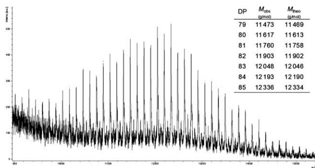
**Fig. 9** MALDI-ToF MS spectrum (main population: Na<sup>+</sup>; minor population: K<sup>+</sup>) of a PLLA sample obtained with  $[L-LA]_0/[8]_0/[^i\text{PrOH}]_0 = 5000:1:50$ , 99% conversion; theoretical molecular weights calculated according to  $\text{DP} \times M_{LA} + M_{i\text{PrOH}} + M_{Na}$ , where DP is the degree of polymerisation,  $M_{LA} = 144.13$ ,  $M_{i\text{PrOH}} = 60.10$  and  $M_{Na} = 23.09$  g mol<sup>-1</sup>.
