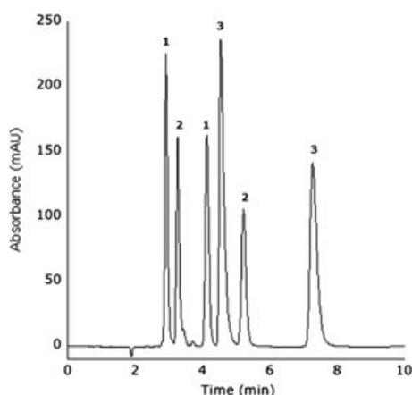
**Fig. 6.** Simultaneous chiral separation of (1) pentedrone, (2) buphedrone and (3) methcathinone. **Conditions:** Column: CHIRALPAK<sup>®</sup> AS-H, mobile phase: hexane/isopropanol/TEA (97:3:0.1), ambient temperature, flow: 1,0 ml/min, UV: 254 nm, injection: 5 $\mu$ l.
