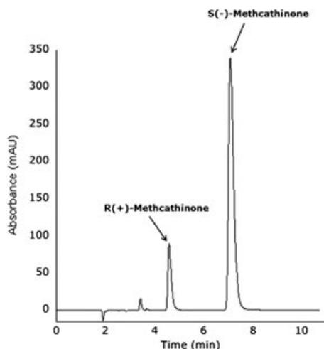
**Fig. 4.** Determination of the enantiomer migration order by means of methcathinone. Conditions: column: CHIRALPAK<sup>®</sup> AS-H, mobile phase: hexane/isopropanol/triethylamine (97:3:0.1), ambient temperature, flow: 1.0 ml/min, UV: 254 nm, injection: 5  $\mu$ l.
