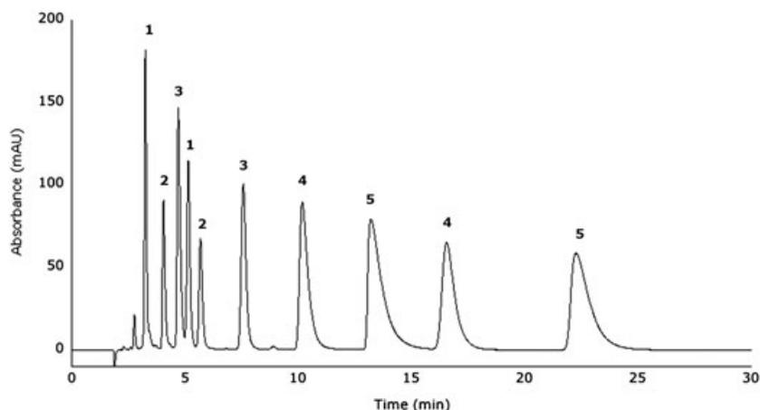
**Fig. 5.** Simultaneous chiral separation of (1) buphedrone, (2) 3-FMC, (3) 4-FMC, (4) methedrone and (5) cathinone. **Conditions:** Column: CHIRALPAK<sup>®</sup> AS-H, mobile phase: hexane/isopropanol/TEA (97:3:0.1), ambient temperature, flow: 1,0 ml/min, UV: 254 nm, injection: 5 $\mu$ l.
