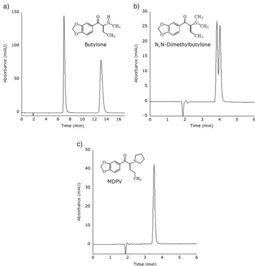
**Fig. 3.** Comparison of the chromatograms of (a) butylone, (b) *N,N*-dimethylbutylone, and (c) MDPV. Conditions: column: CHIRALPAK<sup>®</sup> AS-H, mobile phase: hexane/isopropanol/triethylamine (97:3:0.1), ambient temperature, flow: 1.0 ml/min, UV: 254 nm, injection: 5  $\mu$ l.
