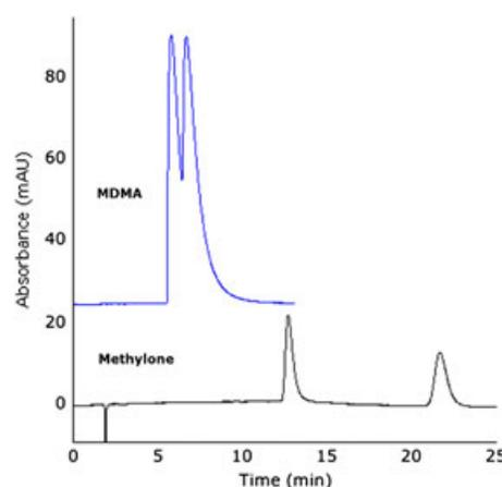
**Fig. 7.** Comparison of the chromatograms of MDMA and methylyone. **Conditions:** Column: CHIRALPAK<sup>®</sup> AS-H, mobile phase: hexane/isopropanol/TEA (97:3:0.1), temperature: room temperature, flow: 1,0 ml/min, UV: 254 nm, injection: 5 $\mu$ l.
