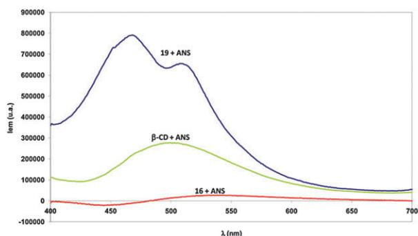
**Fig. 2** Fluorescence emission spectra ( $\lambda_{\text{ex}} = 365 \text{ nm}$ ) of phosphate buffer solutions (pH 7.22) of ANS (0.15 mM) in the presence of  $\beta$ -CD, **16** and **19** (21 mM).
