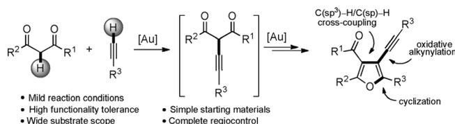
**Scheme 1.** The gold-catalyzed C(sp<sup>3</sup>)-H/C(sp)-H coupling/cyclization/oxidative alkynylation sequence.
