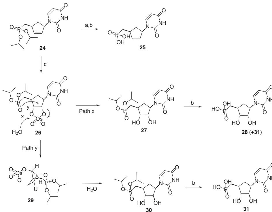
**Scheme 4** a.  $H_2$  (1 atm.), Pd/C (20%), EtOH, 18 h, r.t., 100%; b. TMSBr, MeCN, 16 h, r.t., 20% for compound **25**; 12% for compound **31**, 29% for compound **28**; c.  $OsO_4$ , NMO, acetone,  $H_2O$ , 16 h, 50 °C, 66% overall (22% of **27**, 44% of **30**).
