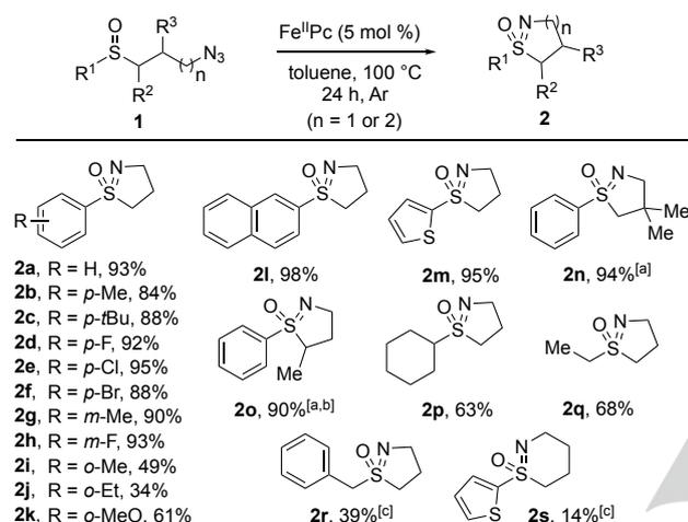
**Scheme 2.** Iron-catalyzed intramolecular imidations of 3-azidosulfoxides **1** (0.2 mmol scale). [a] Use of 20 mol % of Fe<sup>II</sup>Pc at 140 °C. [b] d.r. = 1 : 1. [c] Use of 20 mol % of Fe<sup>II</sup>Pc.
