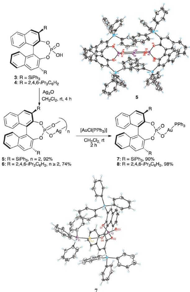
**Scheme 2** Synthesis and structures of Ag(i)–Au(i)–phosphate complexes.
