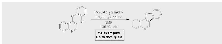
A palladium-catalysed, phosphine-free, direct arylation of 4-phenoxyquinolines in air is described. Using intramolecular direct arylation, the ring-closed products are formed in isolated yields of up to 95%. This approach allows access to a range of benzofuroquinolines, and an array of functional groups on both the quinoline and phenoxy rings is tolerated.
