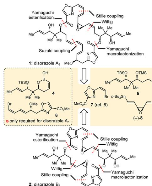
**Figure 2.** Retrosynthetic analyses of disorazoles A<sub>1</sub> (**1**) and B<sub>1</sub> (**2**).
