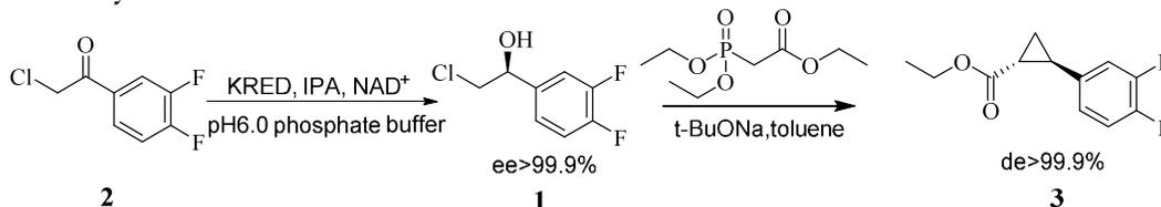
**Scheme 4.** Comparison of the synthetic method of ester **3** from ketone **2**
