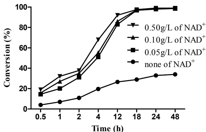
**Figure 8.** The effect of cofactor loading on the influence of conversion
