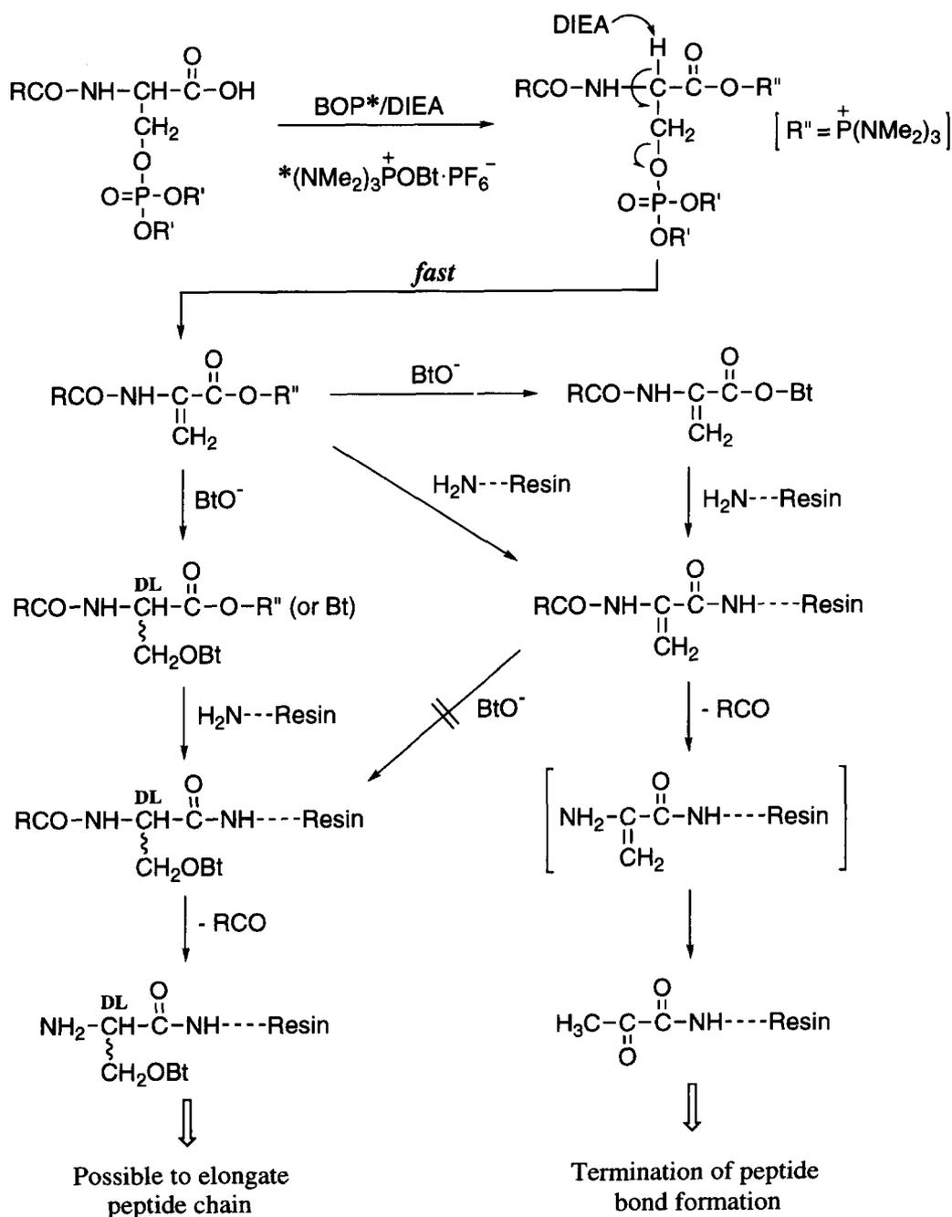
**Figure 1.** Plausible pathways of undesirable reactions occurring through the activation of *O*-(dialkyoxyphosphiny)serine derivatives by the use of BOP for peptide bond formation.
