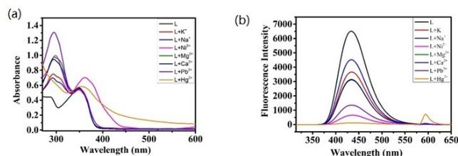
**Figure 2** (a) absorption spectra of compound **3a** ( $c = 2.5 \times 10^{-5}$  M) in MeOH-H<sub>2</sub>O ( $v/v = 1:1$ ) upon addition of several cations. (b) fluorescence emission spectra of **3a** ( $c = 2.5 \times 10^{-5}$  M) in MeOH-H<sub>2</sub>O ( $v/v = 1:1$ ) upon addition of several cations.
