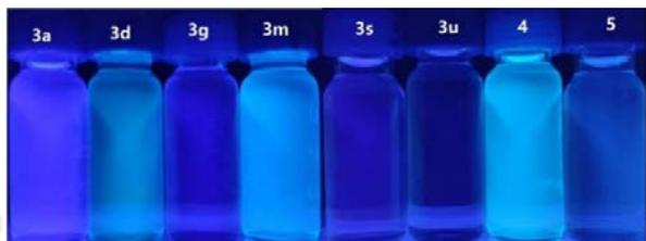
**Figure 1** The fluorescence colours of 2-(quinolin-2-yl)oxazoles in MeOH ( $2.5 \times 10^{-5}$  M) under UV irradiation (365 nm).
