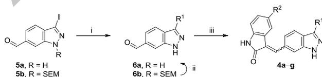
**Scheme 1.** Synthesis of 3-((3-aryl-1H-indazol-6-yl)methylene)indolin-2-one. Reagents and Conditions: (i) arylboronic acid pinacol ester, 10 mol% PdCl<sub>2</sub>(PPh<sub>3</sub>)<sub>2</sub>, 7:1 DME/EtOH, 2 M aq. Na<sub>2</sub>CO<sub>3</sub>, 120 °C; (ii) TBAF, THF, 60 °C; (iii) oxindole, piperidine, MeOH, 60 °C.
