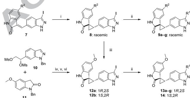
**Scheme 2.** Synthesis of racemic and optically active 2-(3-aryl-1H-indazol-6-yl)spiro[cyclopropane-1,3'-indolin]-2'-ones. Reagents and Conditions: (i) Me<sub>3</sub>SOI, NaH, DMF, rt; (ii) arylboronic acid pinacol ester, 5 mol% Pd(PPh<sub>3</sub>)<sub>4</sub>, 2:1 PhCH<sub>3</sub>/EtOH, 2 M aq. Na<sub>2</sub>CO<sub>3</sub>, 120 °C; (iii) chiral preparative SFC; (iv) NaH, THF, rt; (v) DMSO, *t*-BuOK, THF, O<sub>2</sub> (1 atm), rt; (vi) I<sub>2</sub>, K<sub>2</sub>CO<sub>3</sub>, DMF, rt.
