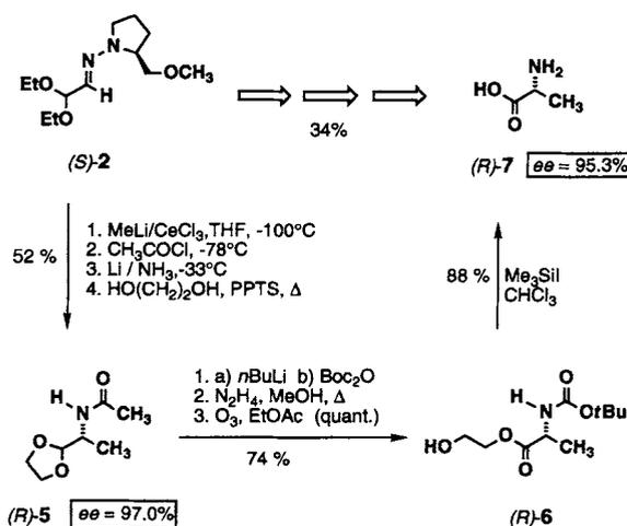
Scheme 2. Enantioselective synthesis of (*R*)-alanine. PPTS = pyridinium *para*-toluenesulfonate. Me<sub>3</sub>SiI was used in excess (3 equiv).
