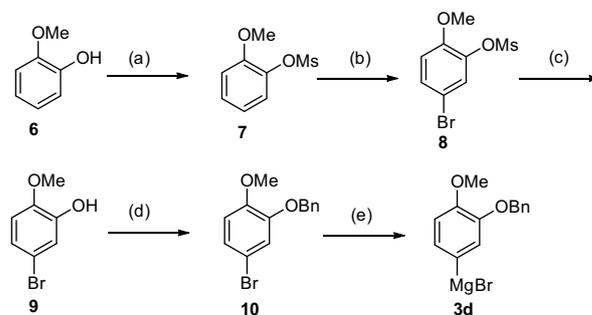
Scheme 2. Preparation of Grignard reagent **3d**. Reagents and conditions: (a) MsCl,  $\text{NEt}_3$ ,  $\text{CH}_2\text{Cl}_2$ , 0 °C, 0.5 h, 96%; (b) NBS, DMF, rt, 24 h, 96%; (c) LDA, THF, 0 °C, 5 min, 91%; (d) BnBr, NaH, THF, 0 °C → rt, 15 h, 99%; (e) Mg, THF, reflux.
