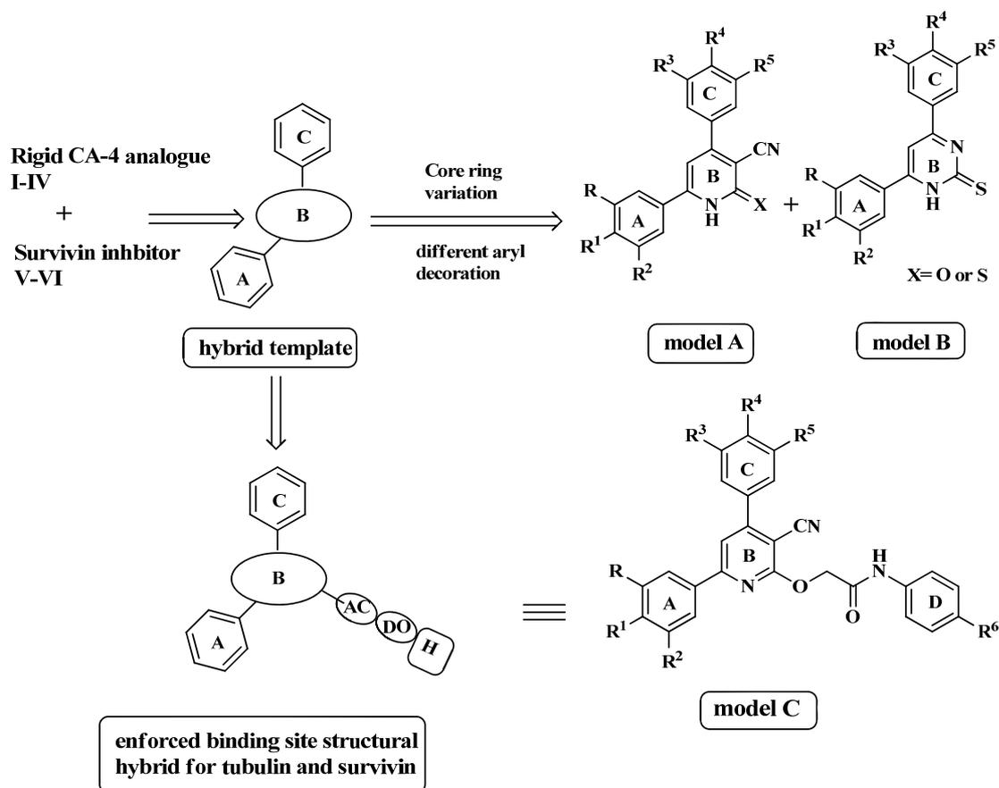
AC=hydrogen bond acceptor,DO=hydrogen bond donor,H, hydrophobic group,A,B,C and D are aryl rings.
