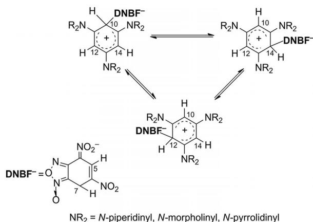
Scheme 2. Proposed mechanism for the reversible dynamic process observed for **WM1–3** in variable-temperature  $^1\text{H}$  NMR experiments.
