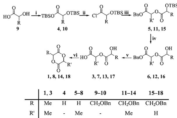
Scheme 4. i) 2.1 equiv. TBSCl, imidazole, DMF. ii)  $(\text{COCl})_2$ , cat DMF, DCM. iii) benzyl (*S*)-lactate/benzyloxy glycolate, pyridine,  $\text{Et}_2\text{O}$ . iv) TBAF/ $\text{HOAc}$ ,  $\text{EtOAc}$ . v) 1 equiv. w/w  $\text{Pd/C}$ , 1,4-cyclohexadiene,  $\text{EtOH}$ . vi) cyanuric chloride, acetone,  $\text{Et}_3\text{N}$
