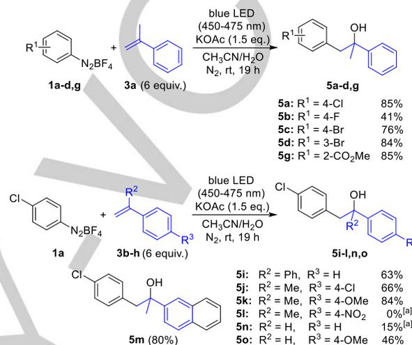
**Scheme 4.** Scope of carbohydroxylation in the presence of potassium acetate. Yields determined after column chromatography; <sup>[a]</sup> Yield determined by <sup>1</sup>H-NMR using 1,4-dimethoxybenzene as internal standard.
