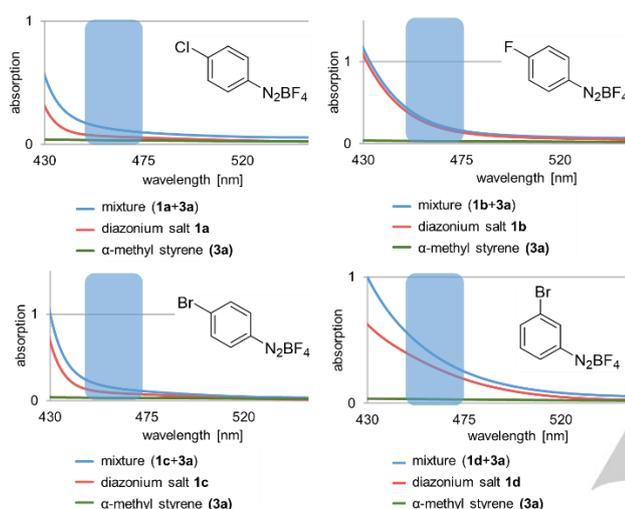
**Figure 2.** UV-Vis spectra of **1a-d**,  $\alpha$ -methylstyrene (**3a**) and the 4 related reaction mixtures.
