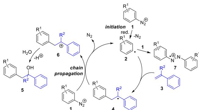
**Scheme 2.** Mechanistic background of the carbohydroxylation of styrenes.
