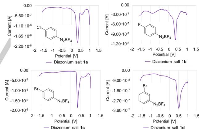
**Figure 4.** Differential pulse voltammetry measurements for **1a-d**.
