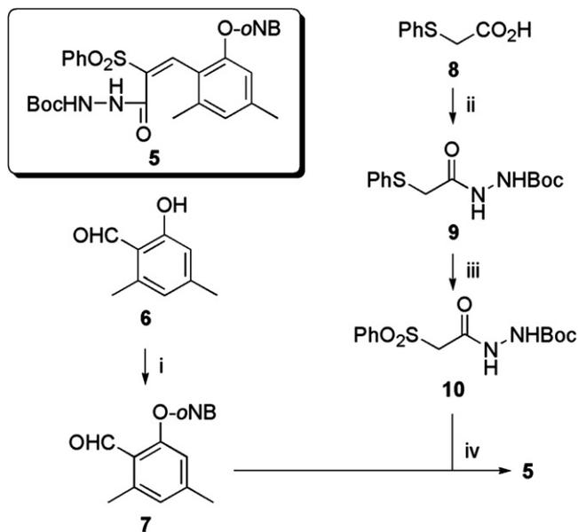
**Scheme 4.** Reagents and conditions: (i) *o*-Nitrobenzyl bromide, K<sub>2</sub>CO<sub>3</sub>, CH<sub>2</sub>Cl<sub>2</sub>, 77%; (ii) H<sub>2</sub>N-NHBoc, *O*-(benzotriazol-1-yl)-*N,N,N',N'*-tetramethyluronium tetrafluoroborate (TBTU), *N,N*-diisopropylethylamine (DIEA), DMAP, CH<sub>2</sub>Cl<sub>2</sub>, 92%; (iii) Oxone<sup>®</sup>, MeOH/H<sub>2</sub>O, 0 °C to room temperature, 74%; (iv) Piperidine, AcOH, toluene, reflux, 85%. (*o*-NB: *o*-nitrobenzyl).
