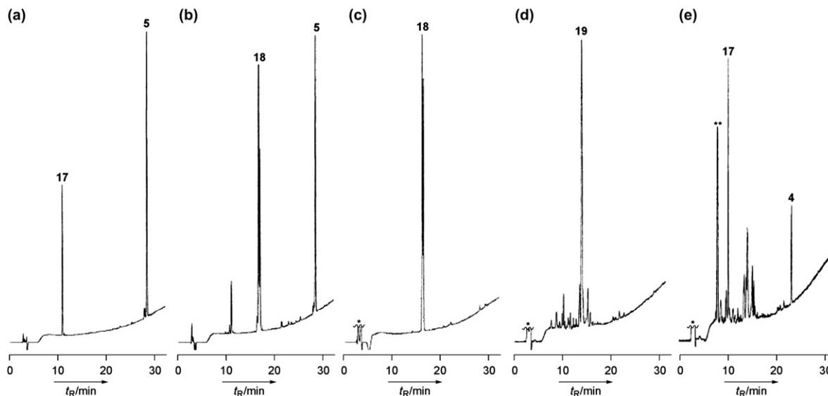
**Fig. 2.** HPLC profiles of catch-and-release reaction of compound 5. Michael addition of peptide 17 to compound 5: (a) 0 h, (b) 24 h. UV-irradiation experiment of compound 18: (c) before UV-irradiation, (d) after UV-irradiation (>365 nm, 5 min), (e) after UV-irradiation (>365 nm, 5 min) followed by incubation at 37 °C in the presence of TCEP for 2 h. Analytical HPLC conditions: linear gradient of solvent B in solvent A, 10–95% over 30 min \*Glutathione. \*\*Non-peptidyl compound.
