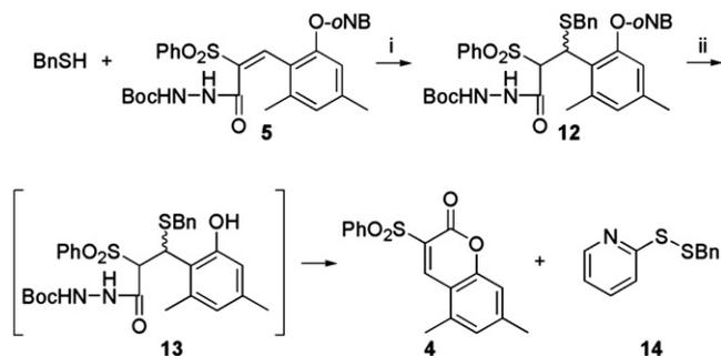
**Scheme 6.** Reagents and conditions: (i) Et<sub>3</sub>N, CH<sub>2</sub>Cl<sub>2</sub>, 82%; (ii) UV-irradiation (>365 nm, 5 min) in MeOH followed by addition of 2,2'-dithiodipyridine and Et<sub>3</sub>N.
