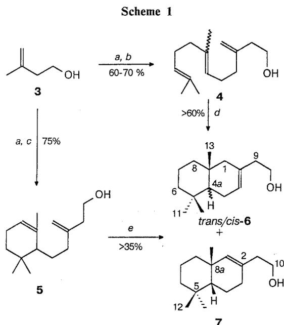
**Reagents and conditions:** *a*, *n*-BuLi/hexane/TMEDA, 25 °C; *b*, geranyl or neryl chloride/THF, -70→25 °C; *c*,  $\alpha$ -cyclogeranyl bromide/THF, -70→25 °C; *d*,  $\text{F}_3\text{B} \cdot \text{OEt}_2$ /hexane, 0→25 °C; *e*,  $\text{F}_3\text{B} \cdot \text{OEt}_2/\text{CH}_2\text{Cl}_2$ , 0→25 °C.
