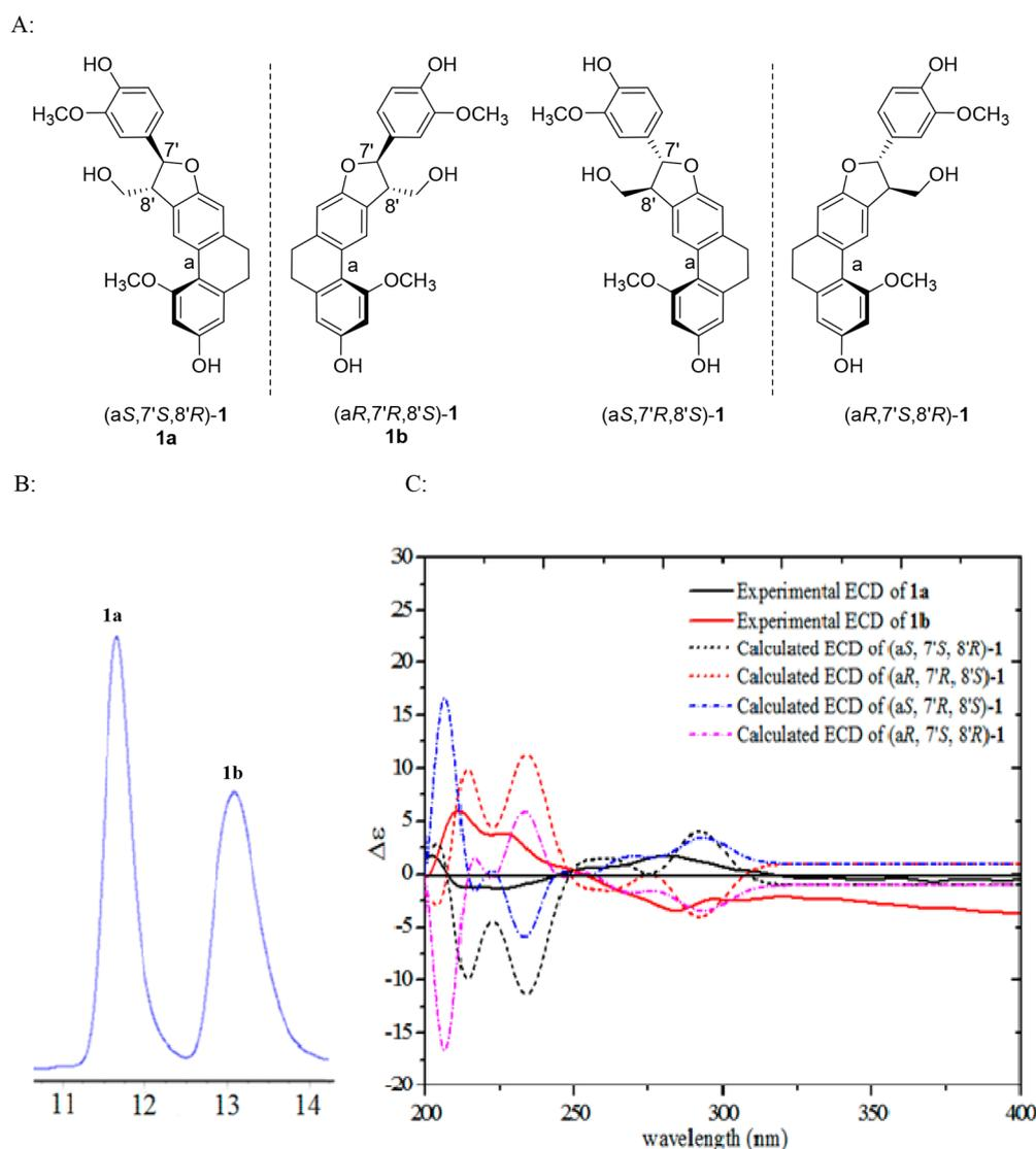
**Figure 5.** Chiral-phase resolution of compound 1. (A) Four possible enantiomers. (B) Chiral-phase HPLC chromatograph. (C) Experimental and calculated ECD spectra.
