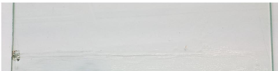
**Figure 7.** Colorless and optically transparent poly(carbohydrate–urethane) coating derived from STC and Priamine 1074/IPDA (40 mol %/60 mol %).
