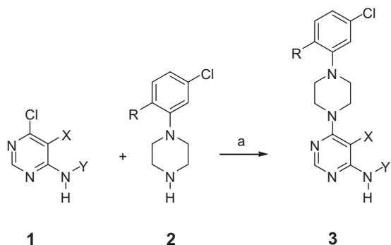
**Scheme 1.** Synthesis of compounds **3** (for detailed structures see Table 1). Reagents and conditions: (a) EtOH, DIEA, 70 °C, 4–15 h, (for **3c**: NMP, DIEA, 180 °C, 16 h; for **3d**: DMSO, DIEA, 140 °C, 15 h).
