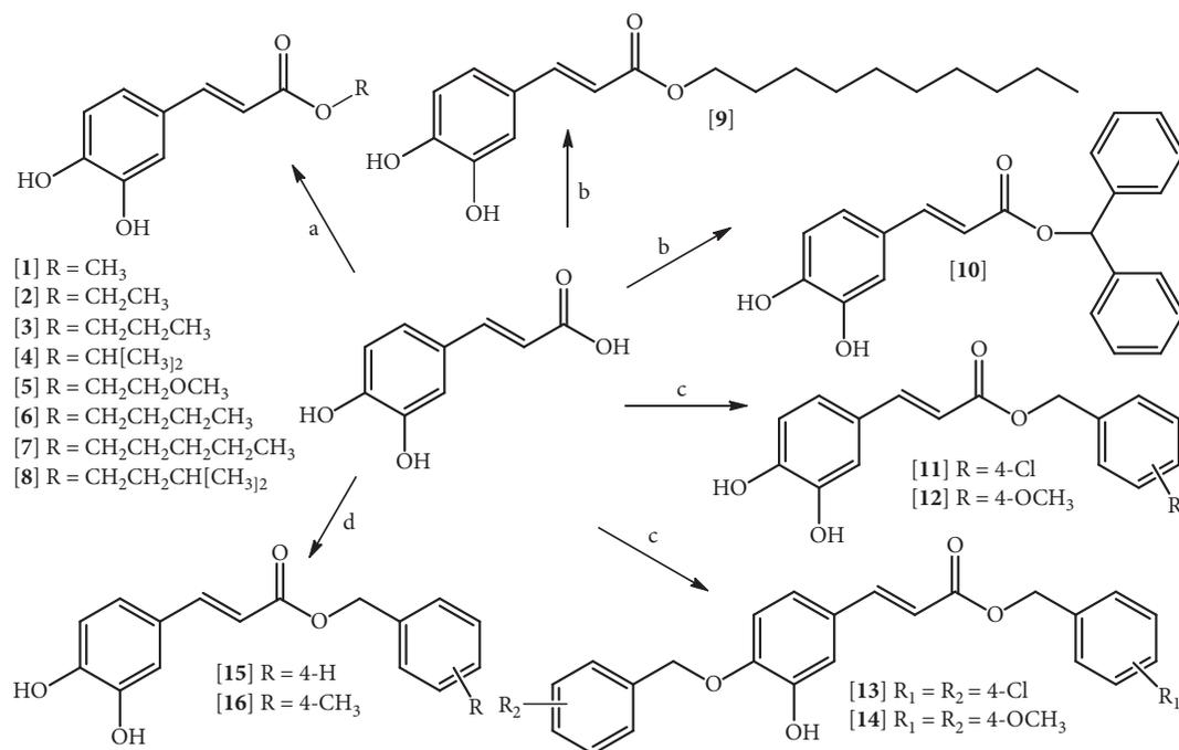
SCHEME 1: Synthesis of the caffeic acid derivatives: (a) ROH, H<sub>2</sub>SO<sub>4</sub>, reflux; (b) Et<sub>3</sub>N, RX, acetone, reflux; (c) DMF, K<sub>2</sub>CO<sub>3</sub>, RX, room temperature; (d) ROH, THF, TPP, DIAD, 0°C to room temperature.
