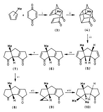
Scheme 1. i, Tetrahydrofuran, room temp., 70%; ii, hv, ethyl acetate, 75%; iii, 530 °C, column packed with quartz chips at 0.1 mmHg, 60%; iv, DBU-CH<sub>2</sub>Cl<sub>2</sub>, reflux, >90%; v, H<sub>2</sub>-10% Pd/C in ethyl acetate, 80%; vi, Ph<sub>3</sub>P<sup>+</sup>-Me I<sup>-</sup>-t-C<sub>5</sub>H<sub>11</sub>O<sup>-</sup>Na<sup>+</sup>, toluene, 30–40%; vii, CH<sub>2</sub>I<sub>2</sub>-Zn/Cu couple, 50%; viii, H<sub>2</sub>-PtO<sub>2</sub> in MeCO<sub>2</sub>H, 3 atm, 60%.
