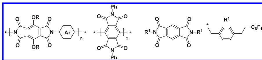
**Figure 1.** PMDI-based materials: polyimide (left),<sup>41</sup> PMDI-based poly(*p*-phenylene) (middle),<sup>40</sup> and PMDI-based *n*-type organic semiconductor (right).<sup>36</sup>
