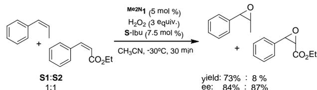
**Scheme 4.** Competitive epoxidation experiment of substrates **S1** and **S2**.
