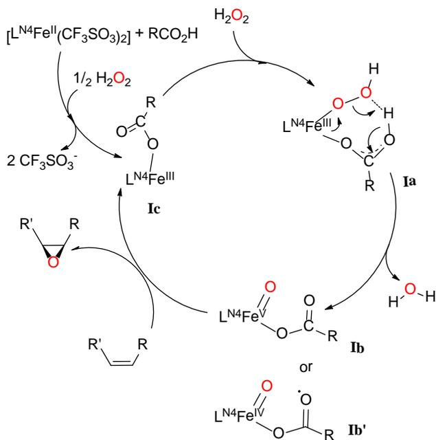
**Scheme 3.** Original mechanistic scheme proposed by Que *et al* for the carboxylic acid assisted O-O cleavage.<sup>15</sup>
