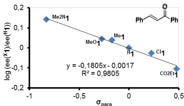
**Figure 1.** Hammett analysis of stereoselectivity as a function of catalyst employed in the epoxidation of **S8** (for analogous analysis with **S1**, **S4** and **S13** see Figures SI.1-SI.2). Catalyst **X1** (1 mol %), AcOH (140 mol %), H<sub>2</sub>O<sub>2</sub> (1.2 equiv) in CH<sub>3</sub>CN at 0 °C. Hammett's values are taken from reference 25.
