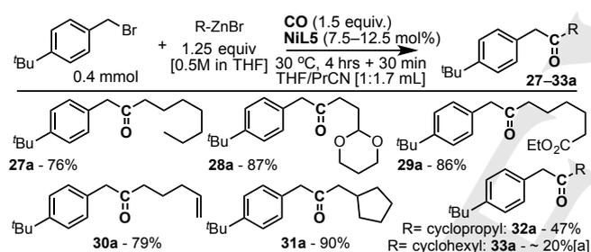
**Scheme 4.** Scope of alkyl zinc reagents. All reactions were conducted in a two-chamber setup, in which CO was released from a solid precursor in one chamber; see Supporting Information for full detail. Yields are isolated and are an average of two separate reactions. [a] Compound not isolated.
