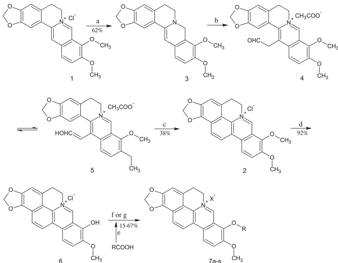
**Scheme 1.** Reagents and conditions: (a) NaBH<sub>4</sub>, 5% NaOH/K<sub>2</sub>CO<sub>3</sub>, CH<sub>3</sub>OH, rt, 2 h; (b) 40% glyoxal, HOAc/CH<sub>3</sub>CN, reflux, 5 h; (c) 2% HCl, rt, 5 d; (d) 20–30 mmHg, 195–210 °C; (e) SOCl<sub>2</sub>, reflux, 2 h; (f) RCOCl, pyridine, CH<sub>3</sub>CN, reflux, 6 h; (g) RX, KOH, DMF, 60 °C, 12 h.
