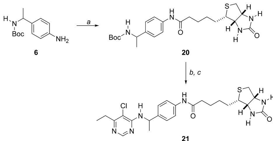
**Scheme 3.** Synthesis of biotin conjugated benzylaminopyrimidine **21**. Reagents and conditions: (a) (+)-biotin, HATU, DIEA, THF, 25 °C, 24 h, 58%; (b)  $\text{CF}_3\text{COOH}$ ,  $\text{CH}_2\text{Cl}_2$ , 25 °C, 3 h, 82%; (c) **4**, DMF,  $\text{K}_2\text{CO}_3$ , 80 °C, 4 h, 45%.
